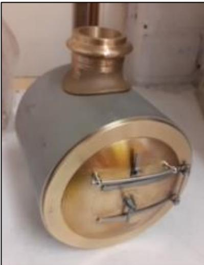
Also made a start on the chimney. Scratched my head for a while as to the best way to hold it whilst boring it to size. In the end I held it by the top 1/4" of the chimney in a 3-jaw chuck getting it to run as true as possible and took very light cuts as it all looked a bit precarious, but it worked. Going to hand file the base of the chimney to fit the smokebox barrel as the casting is not far off from fitting as is.
