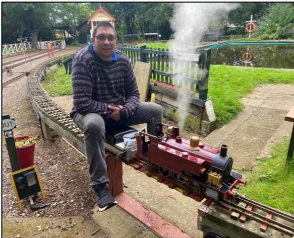
witnessing lack of oil emerging after one lap. This curtailed the test run that day. Subsequent investigation showed the lubricator drive was not working correctly. During cleaning down, it was evident that the blowdown valve was not as tight in its boiler bush as it should be. On opening the valve, the valve body would partially rotate. Not a good thing and one more item to add to the list of problems to be fixed.
