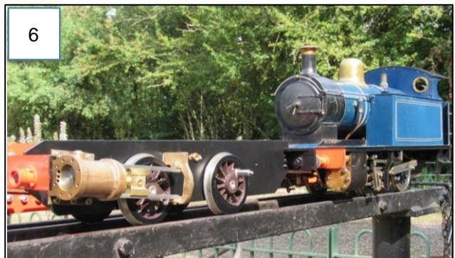
As you can see there is still a lot of work to do, so it remains a Work in Progress. Les told me that he had quite a bit of trouble getting the coupling rods right, so I have now started work on the coupling and connecting rods.
