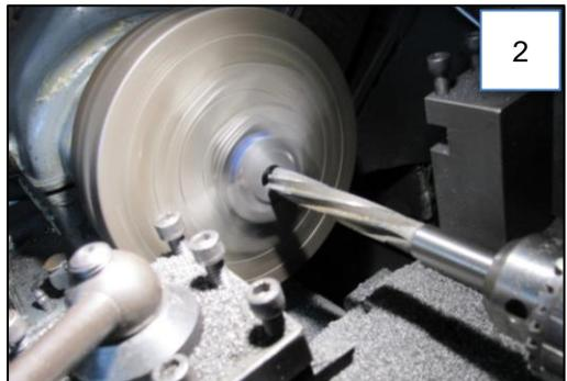
**Picture 2** shows a replacement eccentric being machined.
